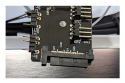
6. If you want to control the fans via your mainboard software, you need to disconnect the ARGB and power connectors of the fans from the fan controller hub.
