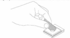
② Completely unfasten the 2 bolts already assembled on the clip and adjust the position to fit the AMD socket. When reassembling the bolt, be sure to assemble only half way of the total length.
